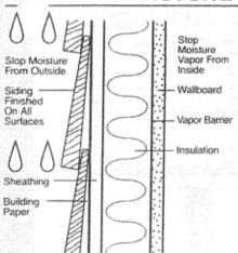
Most siding and trim "problems" and finish "problems" are caused by moisture. All woods shrink as they dry and swell when they absorb moisture. Problems such as checking, buckling, splitting and nail-popping are the result of this dimensional change. Redwood shrinks less than other woods, so it is less likely to have moisture-related problems; as with any wood, some dimensional changes can be expected.
